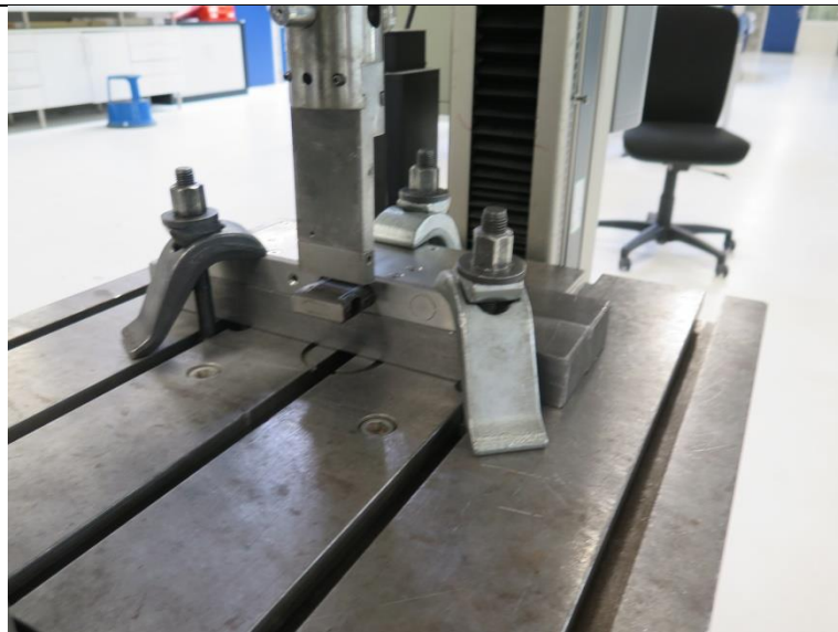
Side load deadbolt after test §5.8.2.1 (supported)
