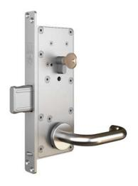
Combination of a mechanical lock with a massive sliding bolt in the door leaf and an electrical striker plate with 2 locking pins in the frame. In the ejected position the bolt is locked in place by these 2 pins, solidly fixing the door leaf to the frame.
